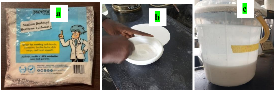
Figure 2: Preparation steps for the bulk solution: (a) raw SDBS powder, (b) powder sampling, and (c) final mixture in the bulk container.
